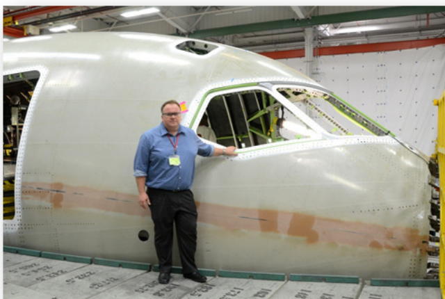
Fwd part of section 41 under construction in Kansas
